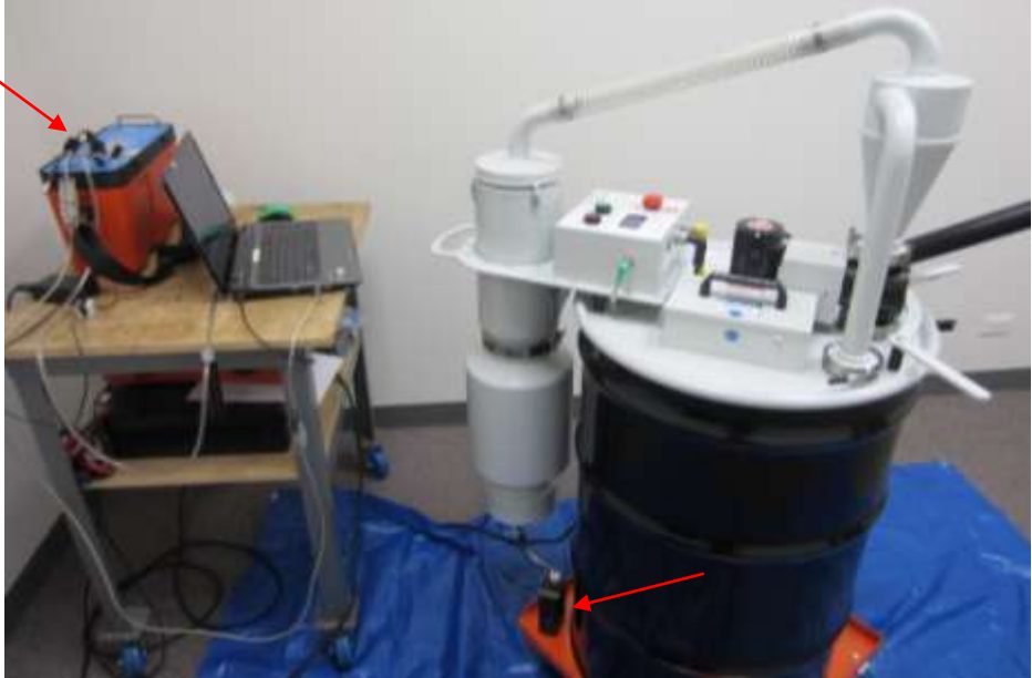
Bulb Eater® 3 testing set-up showing portable battery-powered sampling pump and Mercury Tracker 3000 IP
